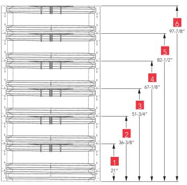
Simply select the number of modules to determine the assembled well height.
