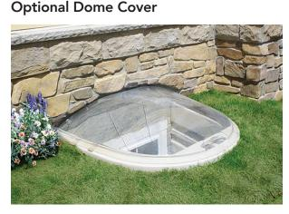
Limits the accumulation of snow, leaves and debris. Constructed of polycarbonate, this high impact cover is UV-resistant and designed for durability and long-life. Dome is designed to withstand a 40 PSF load and is supplied with quick release hold-down clips.
