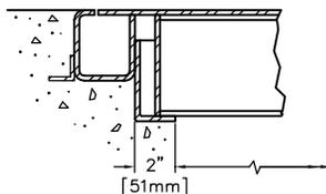
CHANNEL SUPPORT SHELF MUST BE SUPPORTED BY CONCRETE OR STEEL TO CARRY H-20 LOADING
